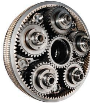
Geared turbofan for new type of aeroengine
